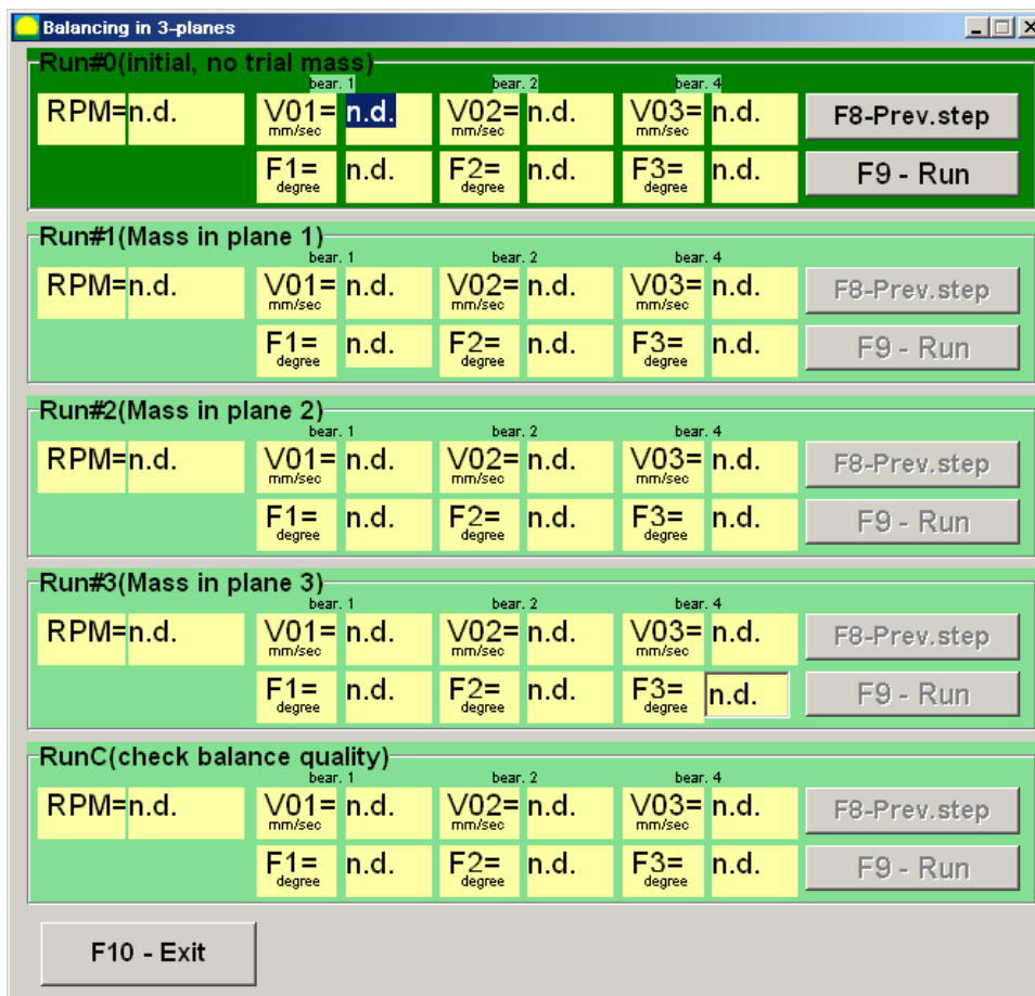
Fig. 7.22. Operating window used for balancing measurements in three planes.
